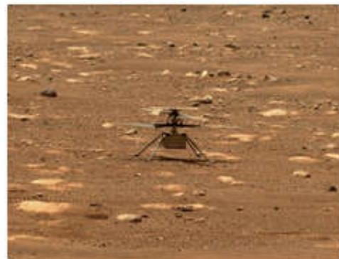
Ingenuity cannot be flown with a joystick, and its flight was not observable from Earth in real time.
